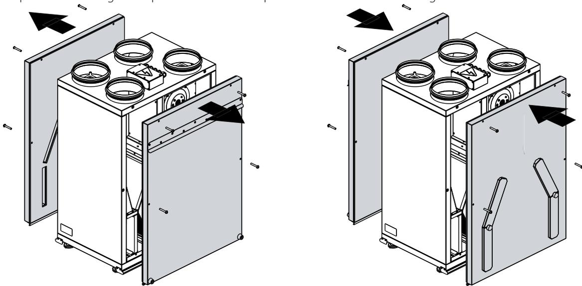
The delivery set includes a label indicating the filter type and the air flow direction. Stick it on a removable plate (only for the KOMFORT EC S(B)250(-E) units).
