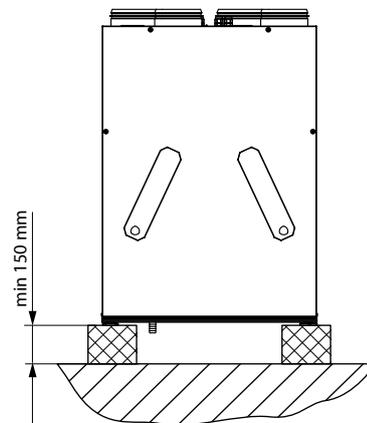
**Note:** mounting is shown by the example of the KOMFORT EC S(B)200(-E) unit.
