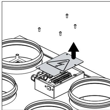
**Access to the terminal box (only for the KOMFORT EC S(B)250(-E) units)**
