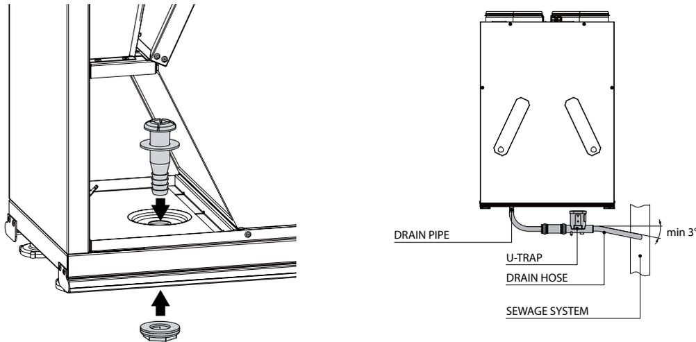
**Note:** installation of the drain pipe is shown on the example of the KOMFORT EC S(B)200 unit.
